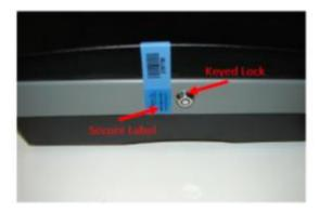
(f) Affix a second label seal over the seam where the top of the unit joins to the base;
