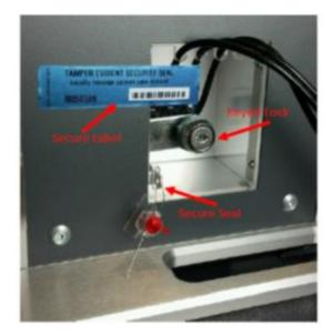
(d) On the left side of the DS450, a clear access door protects the power switch, power cord, network port, and USB port. The access door must be secured using the integrated key lock and a wire or padlock seal. A label seal must also be applied any time the access door is opened and closed again; and
